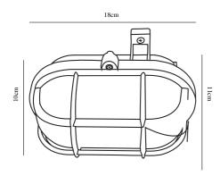
Voltage (V): 230 Volt IP degree: IP44 Maximum bulb wattage (W): 60W Class (Class 1, Class 2, Class 3): Class 2 (Double isolated)
