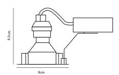
Voltage (V): 230 Volt IP degree: IP23 Maximum bulb wattage (W): 35W Class (Class 1, Class 2, Class 3): Class 2 (Double isolated) Bulb base: GU10 Parallel connection: True
