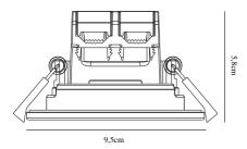
Voltage (V): 230 Volt IP degree: IP20/44 Class (Class 1, Class 2, Class 3): Class 2 (Double isolated) Bulb base: LED Module Parallel connection: True
