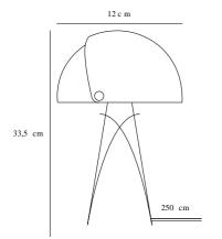
Voltage (V): 230 Volt IP degree: IP20
