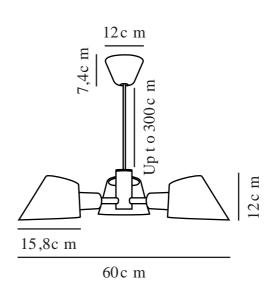
Voltage (V): 230 Volt IP degree: IP20 Maximum bulb wattage (W): 60W Class (Class 1, Class 2, Class 3): Class 2 (Double isolated) Socket type: E27
