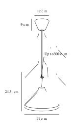
Voltage (V): 230 Volt IP degree if the fixture includes two types of IP degree: IP20 Maximum compatible bulb wattage (W): 40W Class (Class I, Class II, Class III): Class 2 (Double isolated) Lampholder type (eg, E27/E14, etc): E27
