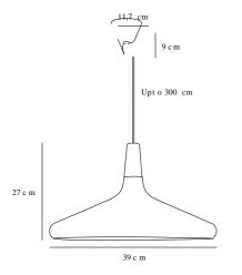
Voltage (V): 230 Volt IP degree if the fixture includes two types of IP degree: IP20 Maximum compatible bulb wattage (W): 40W Class (Class I, Class II, Class III): Class 2 (Double isolated) Lampholder type (eg, E27/E14, etc): E27
