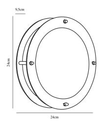
Voltage (V): 230 Volt IP degree: IP54 Maximum bulb wattage (W): 60W Class (Class 1, Class 2, Class 3):
