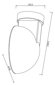
Voltage (V): 220-240 Volt IP degree: IP44 Maximum bulb wattage (W): 10W Class (Class 1, Class 2, Class 3): Class 2 (Double isolated) Socket type: E27 Parallel connection: True
