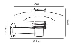
Voltage (V): 230 Volt IP degree: IP54 Maximum bulb wattage (W): 16W Class (Class 1, Class 2, Class 3):
