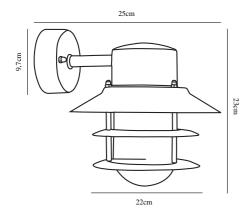
Voltage (V): 230 Volt IP degree: IP54 Maximum bulb wattage (W): 60W Class (Class 1, Class 2, Class 3): Class 1 (Earth contact) Bulb base: E27 Parallel connection: True
