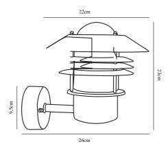
Voltage (V): 230 Volt IP degree: IP54 Maximum bulb wattage (W): 60W Class (Class 1, Class 2, Class 3): Class 1 (Earth contact)
