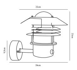
Voltage (V): 230 Volt IP degree: IP54 Maximum bulb wattage (W): 60W Class (Class 1, Class 2, Class 3): Class 1 (Earth contact) Bulb base: E27 Parallel connection: True
