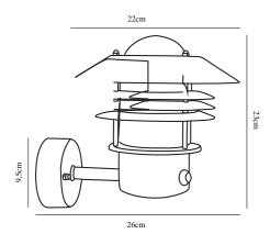
Voltage (V): 230 Volt IP degree: IP54
