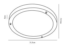
Voltage (V): 230 Volt IP degree: IP44/43 Maximum bulb wattage (W): 2X40W Class (Class 1, Class 2, Class 3): Class 1 (Farth contact)
