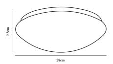
Voltage (V): 230 Volt IP degree: IP44 Class (Class 1, Class 2, Class 3): Class 1 (Earth contact) Bulb base: LED Module
