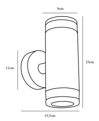
Voltage (V): 230 Volt IP degree: IP44 Maximum bulb wattage (W): 2X28W Class (Class 1, Class 2, Class 3): Class 1 (Earth contact) Bulb base: GU10 Parallel connection: True
