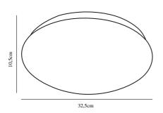
Voltage (V): 230 Volt IP degree: IP20 Class (Class 1, Class 2, Class 3): Class 1 (Earth contact) Bulb base: LED Module
