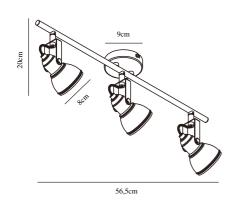
Voltage (V): 230 Volt IP degree: IP20 Maximum bulb wattage (W): 35W Class (Class 1, Class 2, Class 3):
