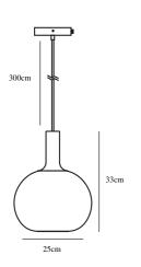
Voltage (V): 230 Volt IP degree: IP20 Maximum bulb wattage (W): 60W Class (Class 1, Class 2, Class 3): Class 1 (Earth contact) Bulb base: E27 Dimmerable: Yes with compatible bulb
