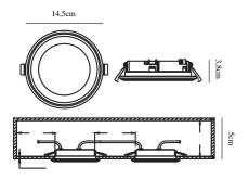
Voltage (V): 230 Volt IP degree: IP20 Class (Class 1, Class 2, Class 3): Class 2 (Double isolated) Bulb base: LED Module Parallel connection: True
