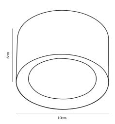
Voltage (V): 230 Volt IP degree: IP20 Class (Class 1, Class 2, Class 3): Class 2 (Double isolated) Bulb base: LED Module Parallel connection: True
