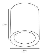
Voltage (V): 230 Volt IP degree: IP20 Class (Class 1, Class 2, Class 3): Class 2 (Double isolated) Bulb base: LED Module Parallel connection: True
