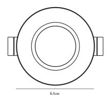
Voltage (V): 230 Volt IP degree: IP65 Class (Class 1, Class 2, Class 3): Class 2 (Double isolated) Bulb base: LED Module Parallel connection: True
