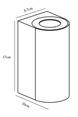
Voltage (V): 230 Volt IP degree: IP44 Maximum bulb wattage (W): 2X28W Class (Class 1, Class 2, Class 3): Class 1 (Earth contact) Bulb base: GU10 Parallel connection: True
