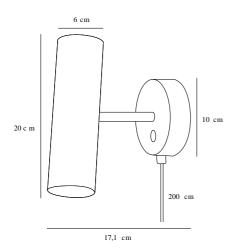
IP degree: IP20 Maximum bulb wattage (W): 8W Class (Class 1, Class 2, Class 3): Class 2 (Double isolated)
