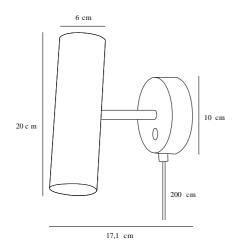
Voltage (V): 230 Volt IP degree: IP20 Maximum bulb wattage (W): 8W Class (Class 1, Class 2, Class 3): Class 2 (Double isolated) Bulb base: GU10 Dimmerable: False Switch placement: On wall base
