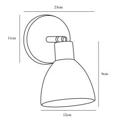
Voltage (V): 230 Volt IP degree: IP20
