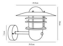
Voltage (V): 230 Volt IP degree: IP54 Maximum bulb wattage (W): 60W Class (Class 1, Class 2, Class 3): Class 2 (Double isolated) Bulb base: E27 Parallel connection: True
