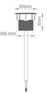
Supplied housing for ground fitting Cut out size: Dia 39mm Mininium deep: 90mm
