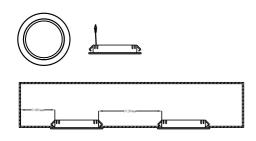
Voltage (V): 12 Volt IP degree: IP20/23 Class (Class 1, Class 2, Class 3): Class 3 (12V) Bulb base: LED Module Switch placement: On the cable Parallel connection: False
