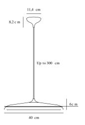
Voltage (V): 230 Volt IP degree: IP20 Maximum bulb wattage (W): 24W Class (Class 1, Class 2, Class 3): Class 2 (Double isolated) Bulb base: LED Module Dimmerable: True
