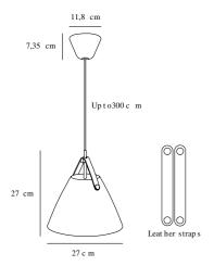
Voltage (V): 230 Volt IP degree: IP20
