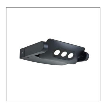
Sigmund has been designed to exploit the benefits of LED lighting characteristics to their maximum. The Sigmund series features a 3 or 6 light fitting, with each bank of 3 LED modules being rotatable by 320 degrees. They are constructed from die-cast aluminium and finished in graphite powder coating. IP65 rated.
