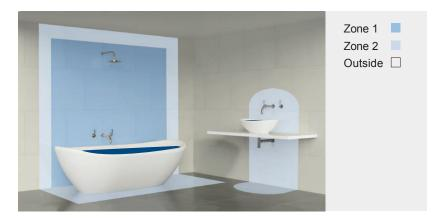
Zone 1 - Above the bath or shower to a height of 2250mm. All lights fitted within this area must be a minimum of IP44 rated. Where a shower head is above the bath IP65 should be used. Lights must be protected by a 30mA RCD if supplied at mains voltage.
