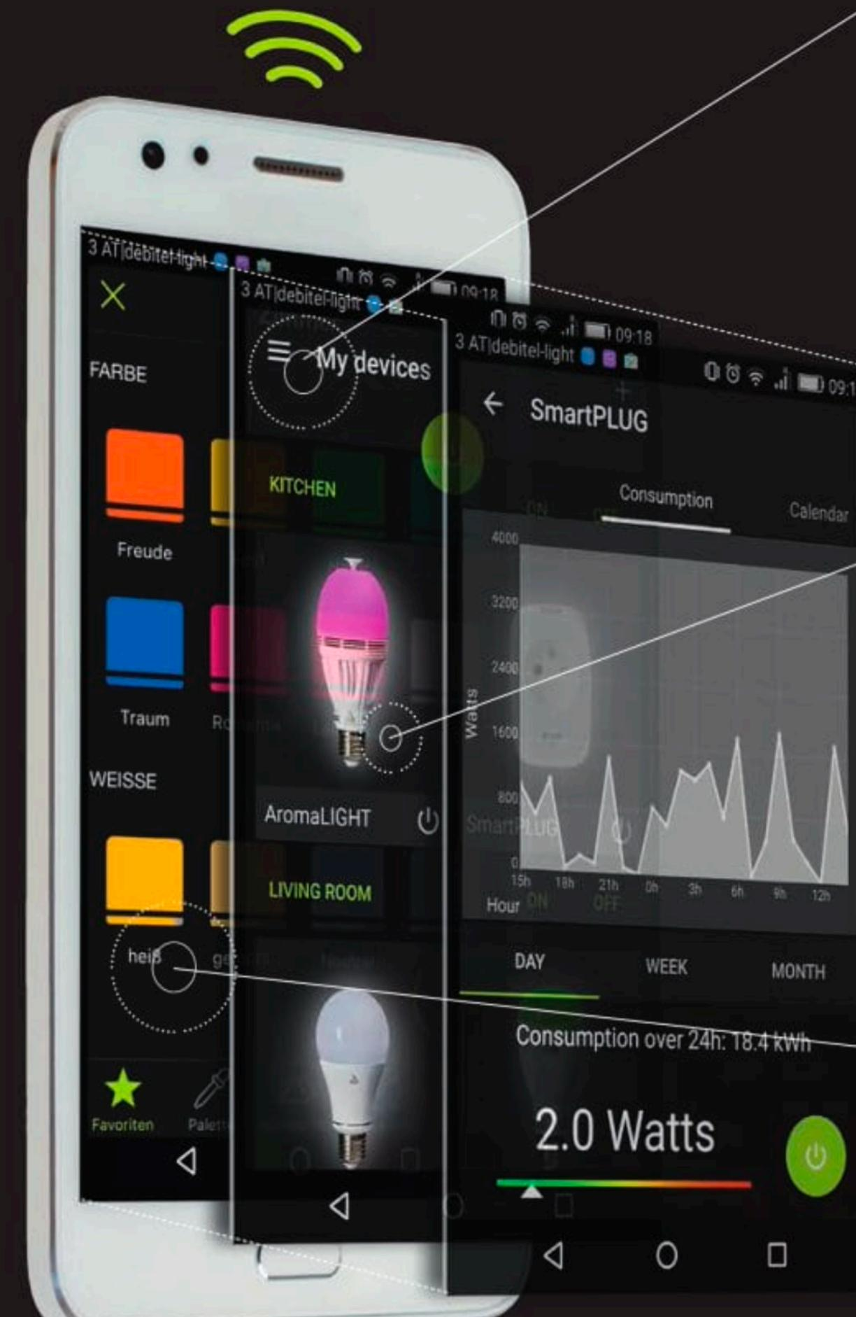
The App permits simple configuration of the network on different levels: from individual lamps to groups. New devices are recognised automatically and can be added to the network on request.
