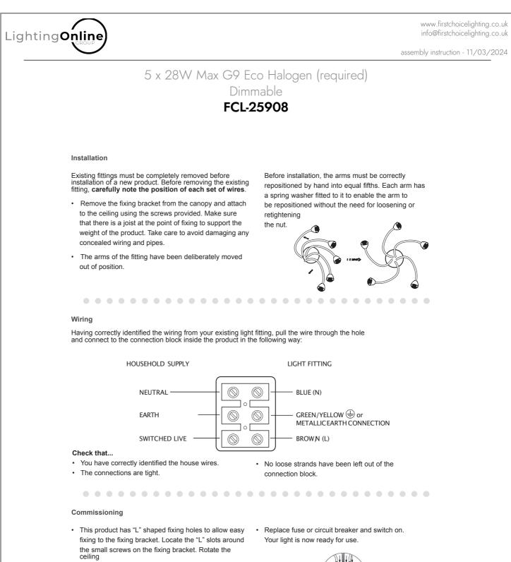
cover to attach the product to the strap. Tighten the screws to secure. Take care not to trap any wiring.
