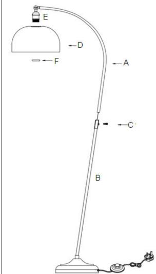
Step 1: Insert the pole A to the pole B and secure them by screwing the threaded nut C.
