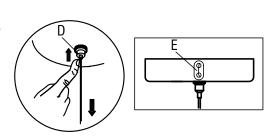
5. Support your fitting and connect the house wiring to the terminal block – see expanded wiring details below. **NOTE: This is a Class II fitting and must NOT be earthed.** Ensure no loose strands are left out of the connection block.
