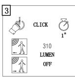
After mode 2, press the switch to change to mode 3. Product will be 310Lm when motion is detected and will turn off after 25 seconds.
